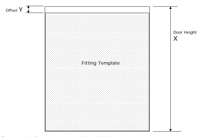
The amount of offset, Y, depends on the height of the fascia door and can be calculated as: -
