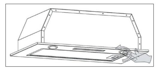
Press gently on the underside of the bulb that needs to be replaced and twist anticlockwise to release.
